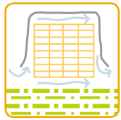
Ventilation under presenning
