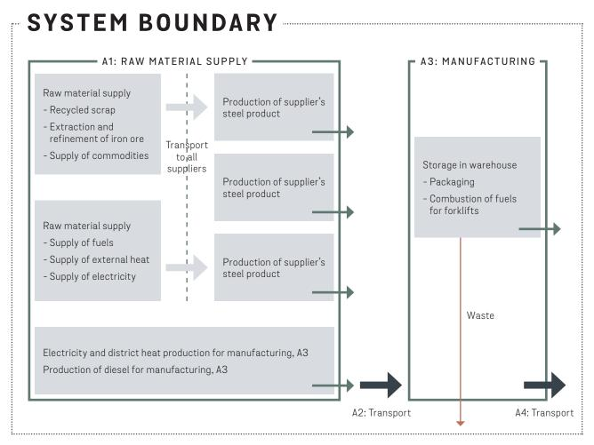
Figure 3. Simplified process tree.
